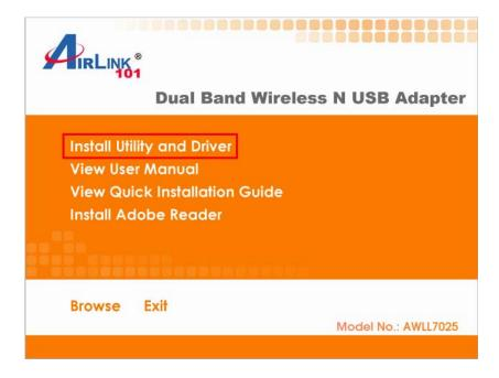
**Note:** If the Autorun screen doesn't appear automatically go to **Start**, **Run**, and type **D:\Utility\Setup.exe** (where **D** is the letter of your CD drive) and click **OK**.
